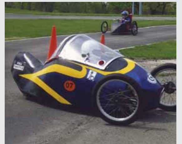
The sporty third-generation "Biodiesel Bomber" competed at the Super Mileage Vehicle Competition in Warrensburg and won the People's Choice, Sportsmanship and Engineering Awards. The vehicle was powered by biodiesel fuel processed from waste oil from the JBS kitchen.
